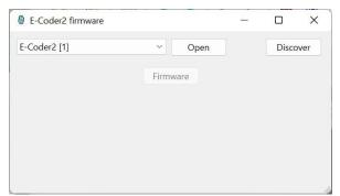
2. Press the Discover button, you'll see a connected to PC E-Coder2 panel. Then Press the Open button.
