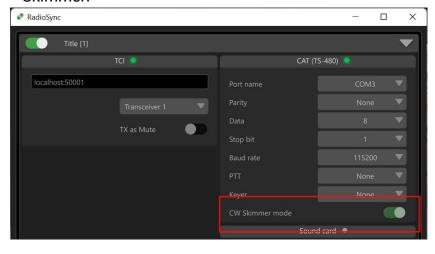
The tuning frequency displayed in the CW Skimmer corresponds to the center frequency of the panorama in the ExpertSDR3. The correct settings in the CW Skimmer: SoftRock-IF, the control works through OmniRig.
