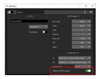
• From now on you can select different devices for RX and TX audio in RadioSync.
