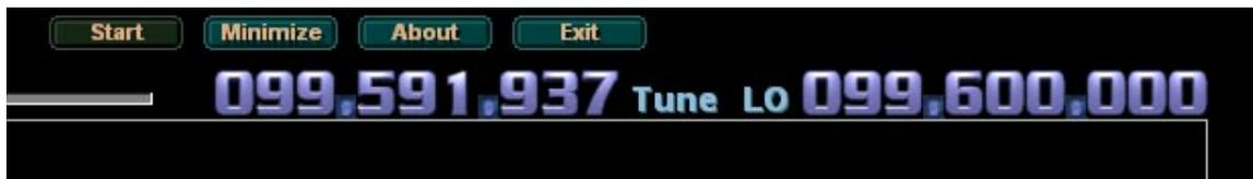
Remember, the centre frequency of the FCD is that shown in Satcontrol’s window. Signals at this frequency appear at the centre of the spectrum display in WRPlus.
