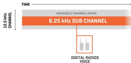
Splits a frequency band into narrow sub-channels and does not use the full capacity of the entire 12.5 kHz channel. As a band narrows, there is greater risk of interference, reduced sensitivity and potentially reduced range resulting in overall reduced performance quality. Relicensing or rebanding is necessary, adding more cost to implement.
