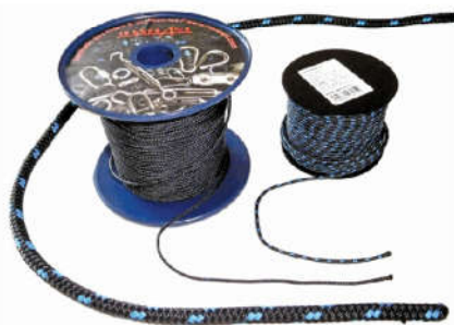
Figure 10 — Mastrant antenna guy ropes are available in a variety of sizes, and here are just a few. The large spool is 100 meters (330 feet) of 2-millimeter M rope, while the smaller spool is 31 meters (102 feet) of 3-millimeter P rope. The larger piece is 10-millimeter P rope.
