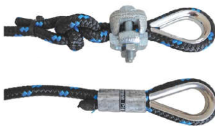
Figure 13 — 10-millimeter rope with fist grip (top) and factory installed thimble with compression fitting (bottom).
