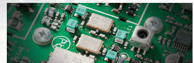
3 kHz and 15 kHz Roofing Filter
