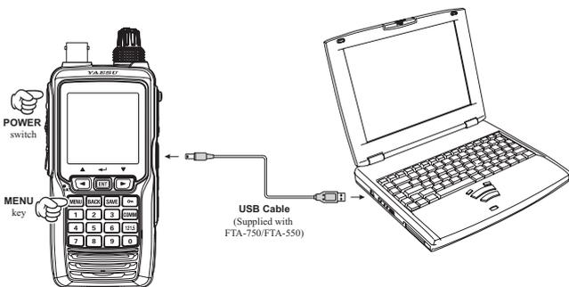
4. Press and hold the [MENU] key while turning the transceiver on, to enter the programming mode.
